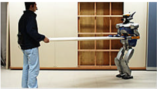
Figure 3: KAWADA Japan developed a humanoid robot for panel assembly. This robot is an example of what is possible with the new technologies, including compactness, interactivity, manoeuvrability and limited weight.
